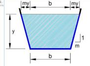
As a civil engineer, you must design a trapezoidal open channel to carry irrigation water. The channel with the minimum "wetted" perimeter is the best hydraulic cross section with the same area of flow since lining and maintenance expenses will reduce substantially.
