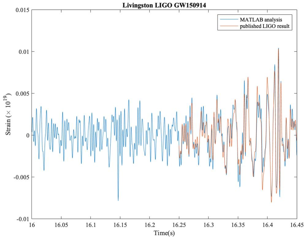
Notice the raw strain levels were 5-8 units and we are looking at .005 or  $6e-4$  of the raw amplitudes. The nature of the filters used may account for the differences.
