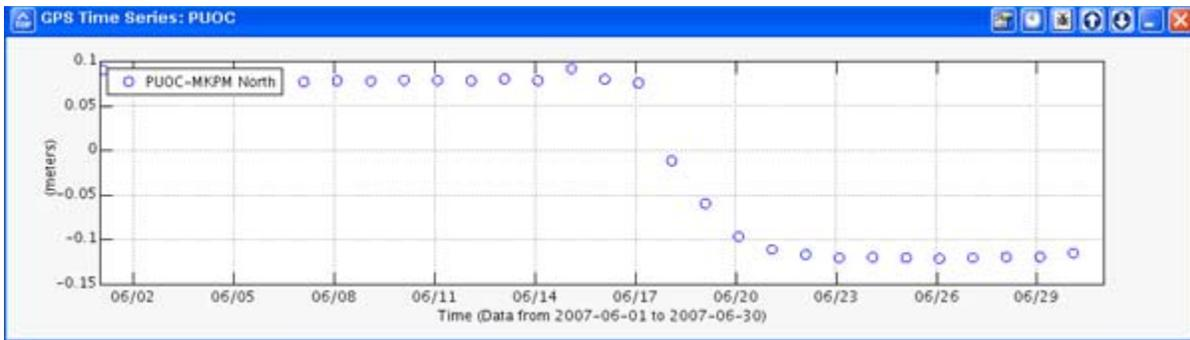
The time series above depicts northward motion of the PUOC GPS station, located on the north rim of Pu'u 'Ō'ō crater, during June 2007. Starting on about June 17, the station began to move south as Pu'u 'Ō'ō deflated and the crater floor collapsed in response to the interruption in magma supply. The motion continued until at least June 23.
