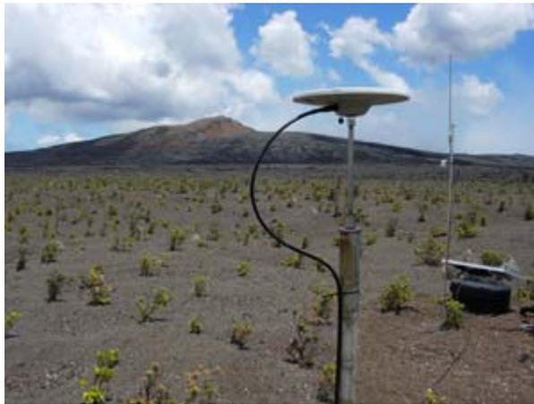
**GPS station KAMO, with Pu'u 'Ō'ō in the background. The GPS antenna is in the foreground, with the solar panel, electronic box, and telemetry mast, and telemetry antennas at right. (2007/08/10)**
