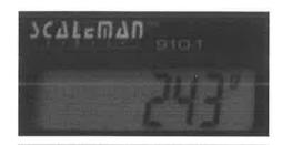
The scale reading is rounded to the nearest gram. The actual reading could be anywhere between 242.5 and 243.5 grams.
