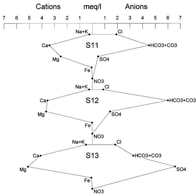
Figure 4. Stiff diagrams for soil and ground-water samples.
