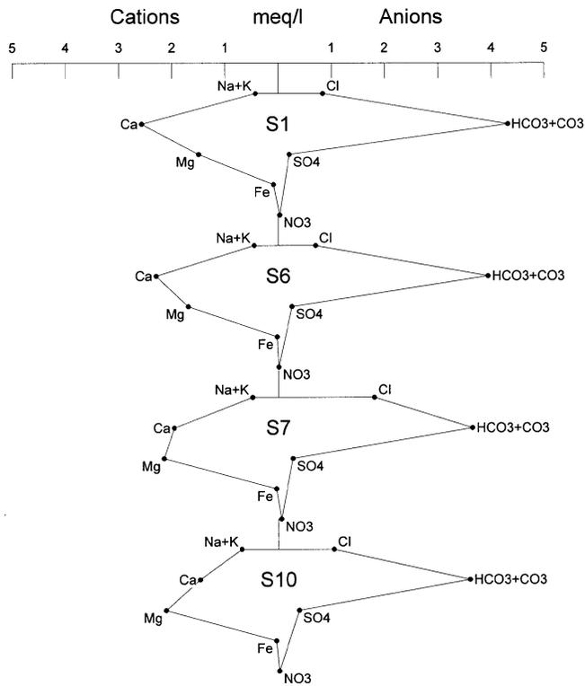
Figure 2. Stiff diagrams for flowing surface water samples.
