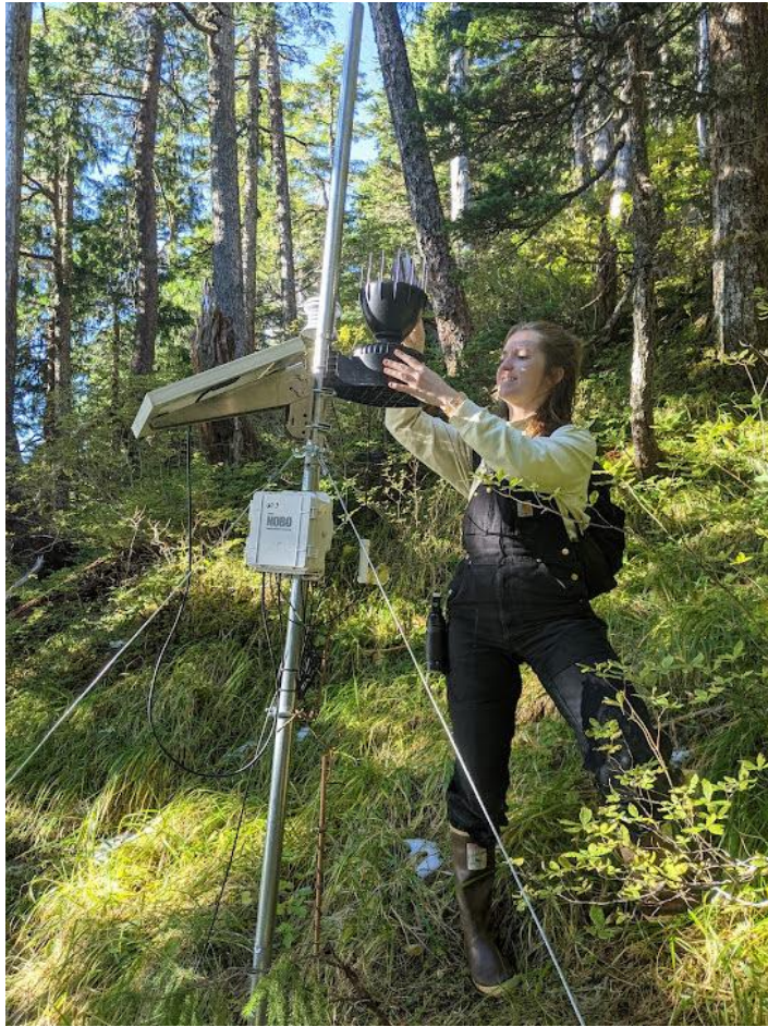
Jacyn Schmidt adjusting the rain gauge on a hydrologic monitoring system that also includes monitors soil moisture using soil conductivity and pressure within a well.
