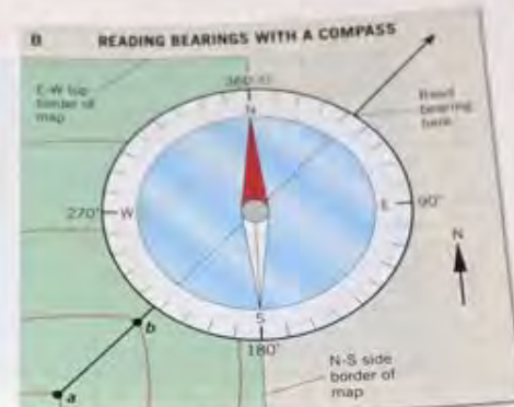
Figure 9.5 How to determine the bearing between two points on a map. A. Bearing from point a through b on a map, determined using a protractor. Center the bearing protractor where a north-south meridian near the points intersects the line from a through b . B. Align the protractor with the meridian. Measure the azimuth clockwise from north to the line from a through b . The range of possible bearing azimuths is from 0 to 360°. B. You can use a compass as a protractor. Align the north-south axis of the compass ring with the meridian, and place the center pivot of the compass at the intersection of the bearing line and the meridian.
