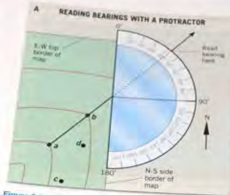
Figure 9.5 How to determine the bearing between two points on a map. A. Bearing from point a through b on a map, determined using a protractor. Center the bearing protractor where a north-south meridian near the points intersects the line from a through b . B. Align the protractor with the meridian. Measure the azimuth clockwise from north to the line from a through b . The range of possible bearing azimuths is from 0 to 360°. B. You can use a compass as a protractor. Align the north-south axis of the compass ring with the meridian, and place the center pivot of the compass at the intersection of the bearing line and the meridian.
