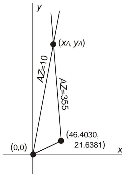
**Figure 6. Graph showing information to determine position of  $A$  using linear equations.**
