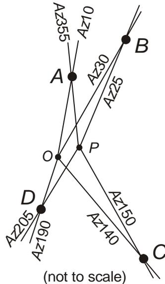
**Figure 9. Sketch showing sightings to locate the four vertices of a quadrilateral from a single baseline ( $OP$ ).**
