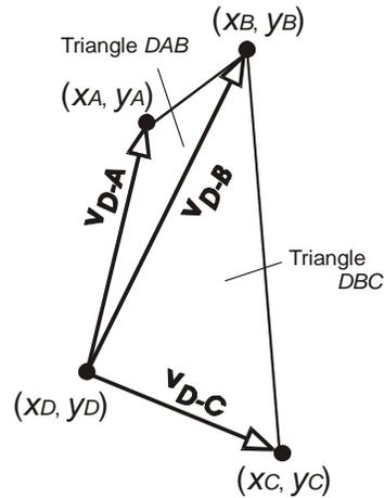
**Figure 11. Sketch showing vectors to find the area of the quadrilateral using the cross-product (Equations 21 and 22).**
