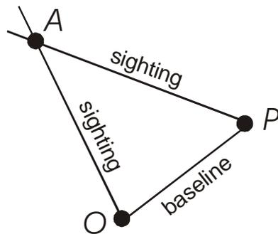
**Figure 1. Definition diagram for the essential ingredients of a triangulation problem.**
