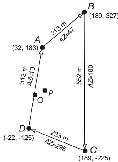
**Figure 17. Diagram of the quadrilateral drawn to scale to check for calculation errors.**
