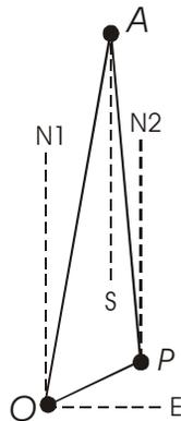
**Figure 3. Map showing angles used in the law of sines to find the position of A. E and S indicate directions to the east and to the south, respectively, and  $N_1$  and  $N_2$  indicate the direction to north.**
