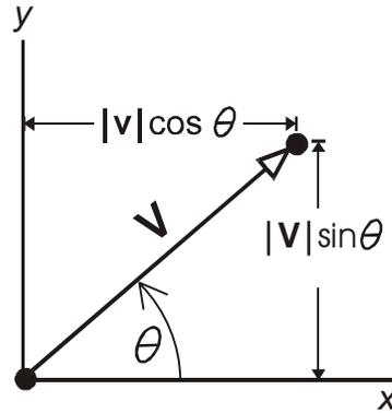
**Figure 5. Sketch showing the components of a vector.**
