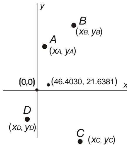
**Figure 10. Sketch showing the coordinates of the end-points of the baseline and the vertices of the problem quadrilateral. Extra digits for  $P$  for purpose of calculation.**
