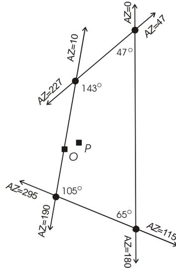
**Figure 18. Diagram used to compare direction information with vertex angles.**
