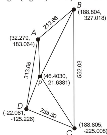
**Figure 19. Diagram used to find the central angles about P and the area of the quadrilateral trigonometrically. Extra digits for purpose of comparison.**
