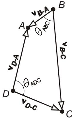
**Figure 13. Sketch showing vectors to find the vertex angles at B and D using the dot product (Equation 26).**
