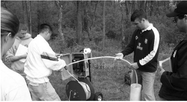
**Figure 2. Introduction to Hydrogeology students at SUNY New Paltz are conducting a pump test at the Institute of Ecosystem Studies (IES) monitoring well site.**
