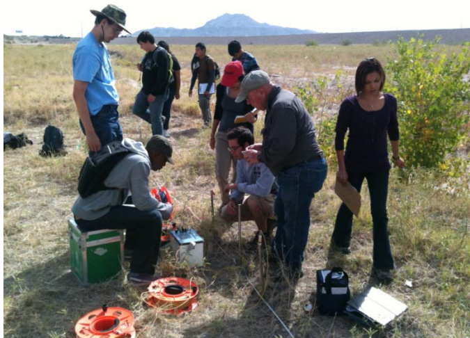
Students in the EPCC GEOL 2407 Geological Field Methods class performing a resistivity profile with students in the UTEP GEOL 4334 Non-Seismic Methods class.
