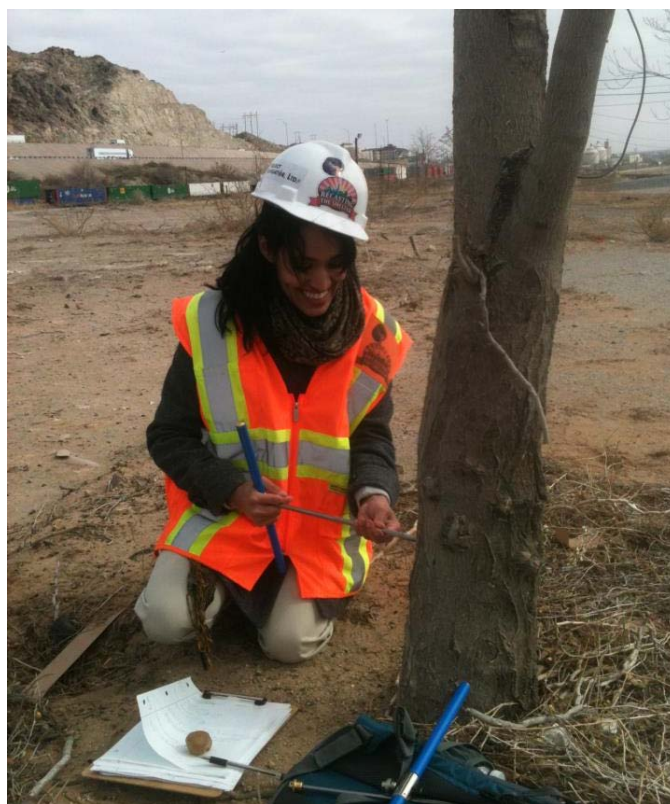
Sandra Garcia EPCC Geological Science major collecting tree core samples at a closed copper refinery for her NSF-funded research. The cores will be analyzed for toxic metals.
