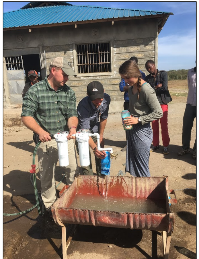
Russ Kohrs, with students, testing their bone char filtration apparatus in Kenya.
