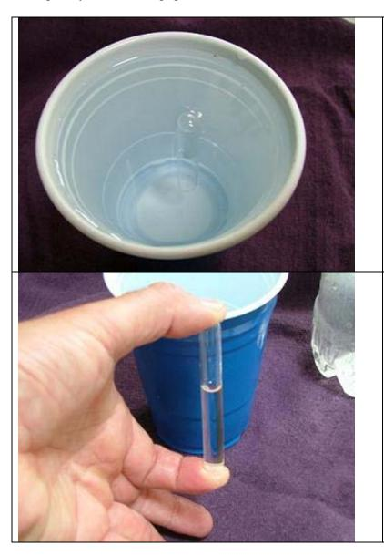
Partially fill a small test tube with water so that when it is inverted and placed in a beaker full of water it barely floats.
