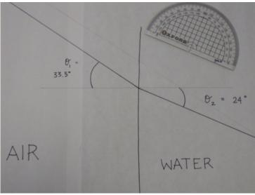
Illustration of steps 12, 13, and 14. The angle of incidence  $(\theta_1) = 33.5^{\circ}$  and the angle of refraction  $(\theta_2) = 24^{\circ}$ . Note that the protractor is just sitting there as a prop. I obviously did not measure the angles from way over there!
