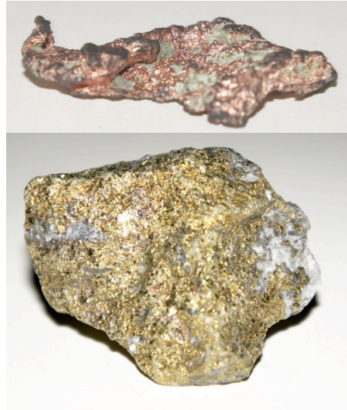
Figure 8. Copper's electrical conductivity and resistance to corrosion make it ideal for electric wiring. Although copper can be found as a pure metal (native copper, upper right ), it is often beneficiated from minerals like chalcopyrite ( \text{CuFeS}_2 , lower right ).
