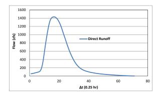
For an observed storm event, direct-runoff hydrograph at 15 mins interval is shown below.
