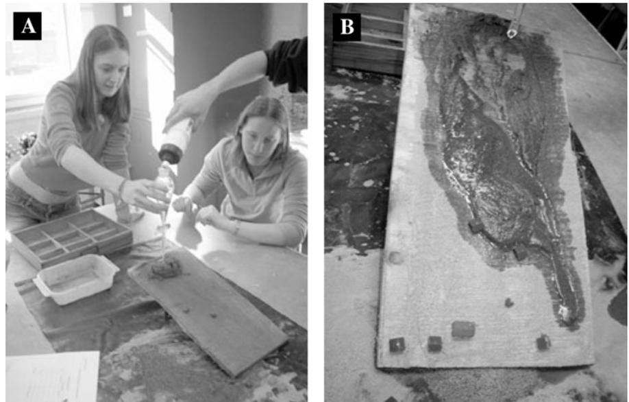
*Fig. 1. Hands-on modelling of mass movements is used as a catalyst for student discussion. (A) Students drip water onto moist sand in order to initiate a flow down the wooden ramp. (B) A flow engulfs local infrastructure (Monopoly houses). Such activities help students build connections between geoscience and their own lives.*
