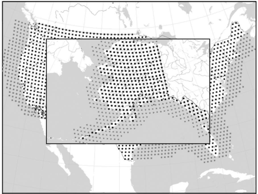
Fig. 3. USArray Bigfoot stations (black dots) and proposed Webfoot offshore ocean bottom seismic array (gray dots), which would move with USArray around the margins of North America are shown. As recommended, Webfoot would consist of ~150 OBS spaced 70 km apart extended ~600 km offshore.
