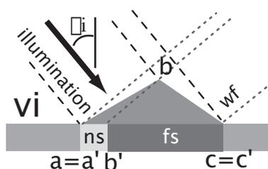
(iv) Left illumination and an asymmetric topographic form with steep slope facing radar results in extreme foreshortening, or "layover". Only the far slope is imaged because b projects to b' and a, projected to a', is lost in extreme foreshortening. Although the near slope is lost to layover, none of the far slope is lost to radar shadow in this case.
