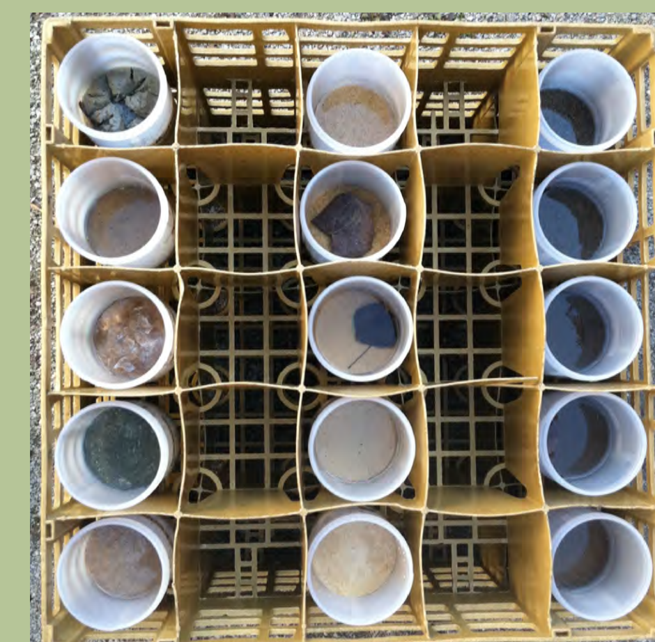
Figure 9: Natural delivery experiment. Samples are exposed for one month then brought inside for counting. Rainwater is also collected and measured.
