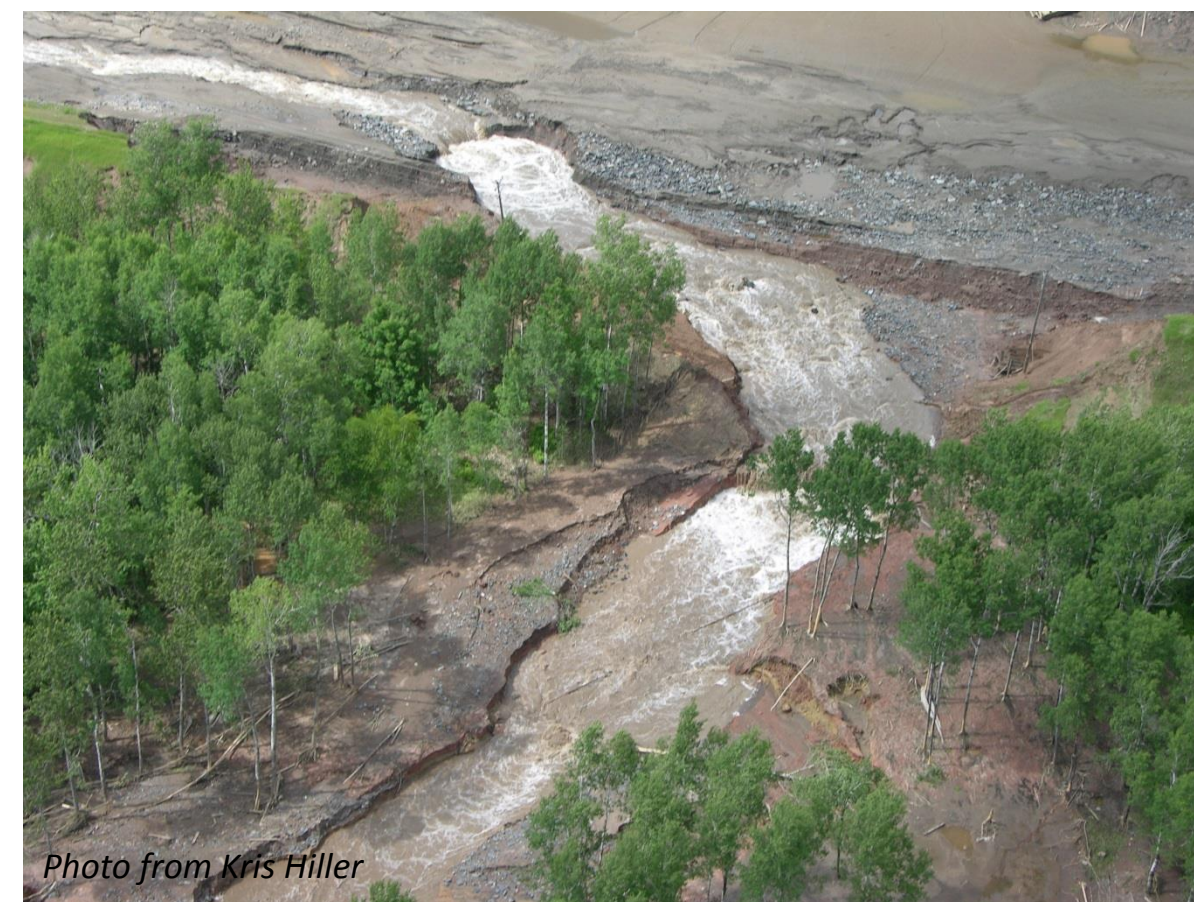
Levee breach as viewed from above (top) and from the ground (left). The failure occurred rapidly, sending a wave of water and sediment downslope.
