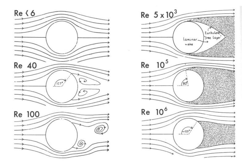
Figure 4.3 Flow patterns around circular cylinders normal to the flow, for Reynolds numbers from less than six to about  $10^6\,\cdot$
