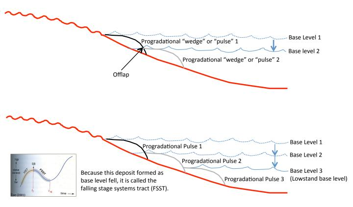
Add erosion to give a more realistic picture of the preserved deposit. Notice that Progradational Pulse 1 has been entirely "cannibalized" and Pulse 2 is mostly gone.
