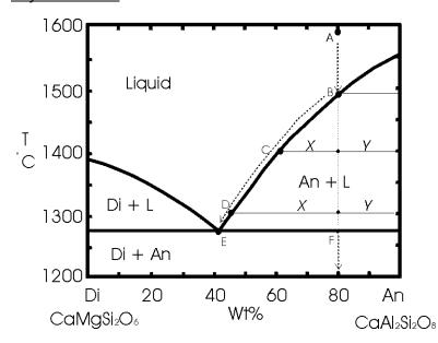
The diagram at left shows what happens to a liquid of composition A as it cools. Composition A is about 80% CaAl<sub>2</sub>Si<sub>2</sub>O<sub>8</sub> - 20% CaMgSi<sub>2</sub>O<sub>6</sub>, abbreviated An<sub>80</sub>Di<sub>20</sub>.
