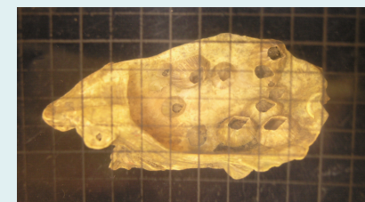
Figure 6. Oyster valve with transparent grid. Grids were used in point counting method to determine extent of Ciona sp. borings and encrustation
