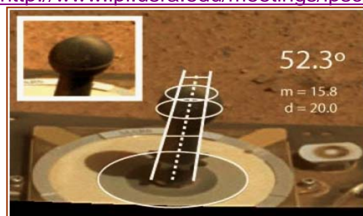
Figure 1. NASA Spirit MER Marsdial color image extracted from the panorama photograph taken from the summit of Husband Hill during sols 583 to 585 (August 24 to 26, 2005). Inset photo shows the reddish brown, apparent dust deposition cap. Image analysis using the elliptical planes shown for the extraction of dust deposition: d = 52.3^\circ from sand ( d = m/d ).
