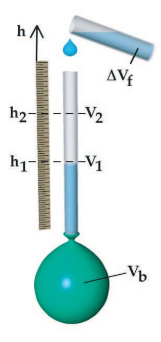
Figure 1: Apparatus to measure specific storage coefficient of a water-filled balloon.
