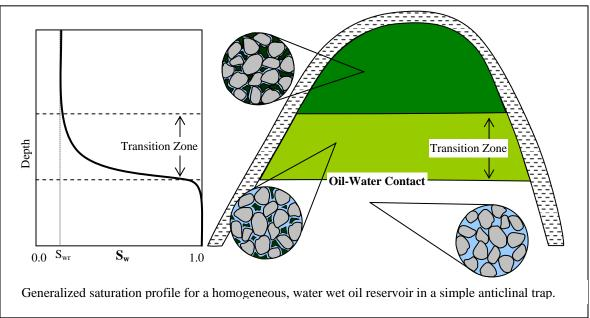
The oil-water contact is defined as the lowest elevation from which oil can be produced. Below the oil-water contact, only 100% water can be produced. A zone of transitional saturations is found above the oil-water contact, from which an increasing proportion of oil can be produced with decreasing depth until the residual (irreducible) water saturation,  $S_{wr}$ , is reached. Above this elevation, oil is the only mobile phase and 100% oil production occurs.
