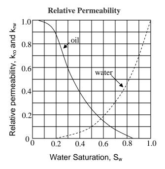
Oil and water relative permeability curves for an oil wet reservoir system (after Craft, Hawkins, and Terry, 1991). At 50% water saturation, the relative permeability to water is approximately 10% and the relative permeability to oil is approximately 25%. Oil permeability is favored because it occupies the center of the pore spaces in a water wet reservoir.
