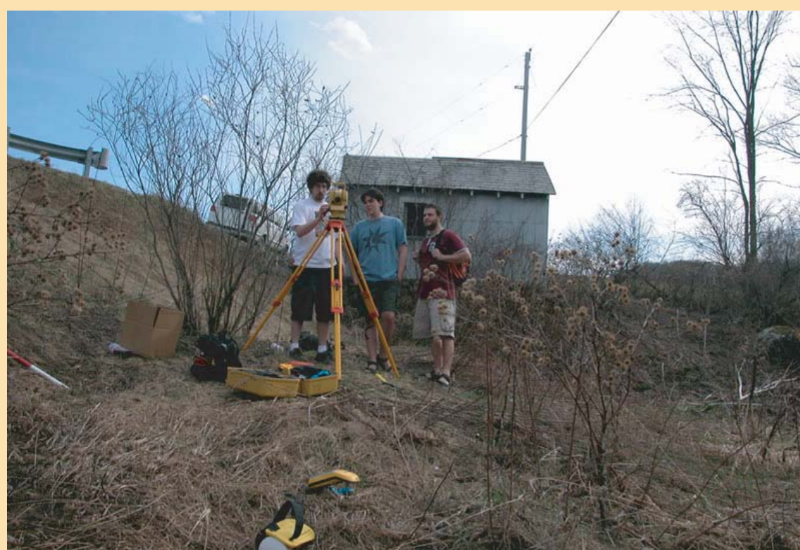
Figure 6: Hydrology and chemistry students collecting survey data for cross sectional profile at Site 3.
