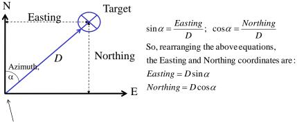
You are here, and you measure a distance D and azimuth  $\alpha$  to the target. We want to convert these to components (yes, this is a vector!), which are the easting and northing coordinates.
