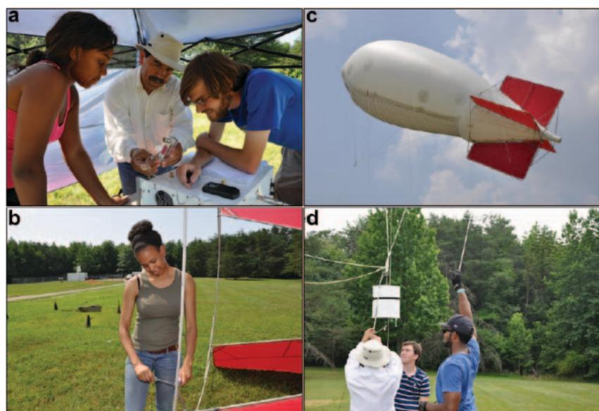
Fig. 1. A group of students in the Underrepresented Geoscience Education (URGE) program prepare equipment (a) to measure ambient levels of air pollutants, assembling fins (b) on a tethered balloon (c) that lifts the necessary instrumentation for their study. (d) Hung from the balloon is a tethered sonde (white cylinder) that houses instruments that determine the vertical distribution of air pollutants and aerosols.
