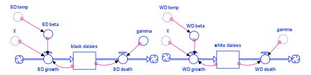
In this graphic, the dependency of BD beta and WD beta on the local temperature has been specified through the addition of the BD temp and WD temp converters.
