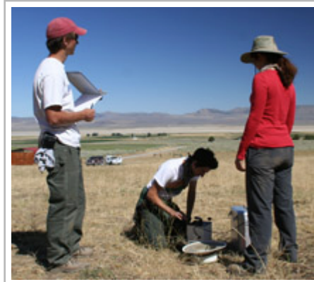
Students measuring gravity and shading the gravity meter in Surprise Valley, California. Created by Anne Egger, Stanford University Details
