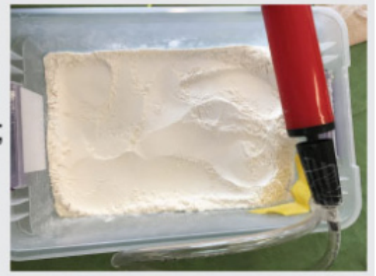
Top: Parts. Center: balloon taped to bottom of plastic tub. Lower: Flour buries the balloon.
