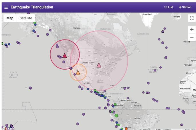
Solution for triangulating the student's 3 seismic stations as derived from IRIS's online app "Triangulation".
