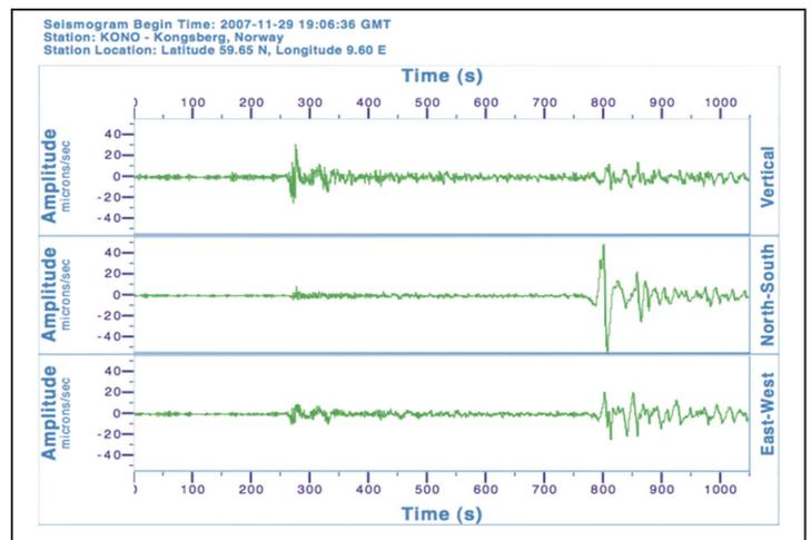
**Figure 2** – Modern seismic stations produce a 3-component seismogram.
