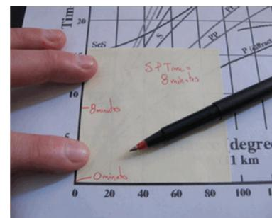
b. Keeping the paper edge parallel with the y-axis, slide the paper to the right and upward. Find the spot in the graph where the marker you created fits between the S and P curves on the travel time curves.
