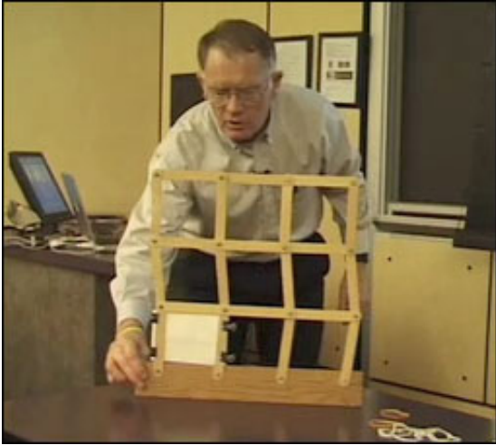
Dr. Robert Butler, University of Portland OR demonstrates structural additions for building strength during an earthquake.
