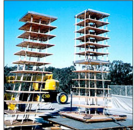
*Base isolation, also known as seismic or base isolation system, is a collection of structural elements which should decouple a structure from the ground. If the ground below a building shifts abruptly to the left as shown in the experimental buildings here, the building with base isolation on the right becomes an inertial mass that stays in the same place during the jolt due to structural elements that decouple it from the earth.*
