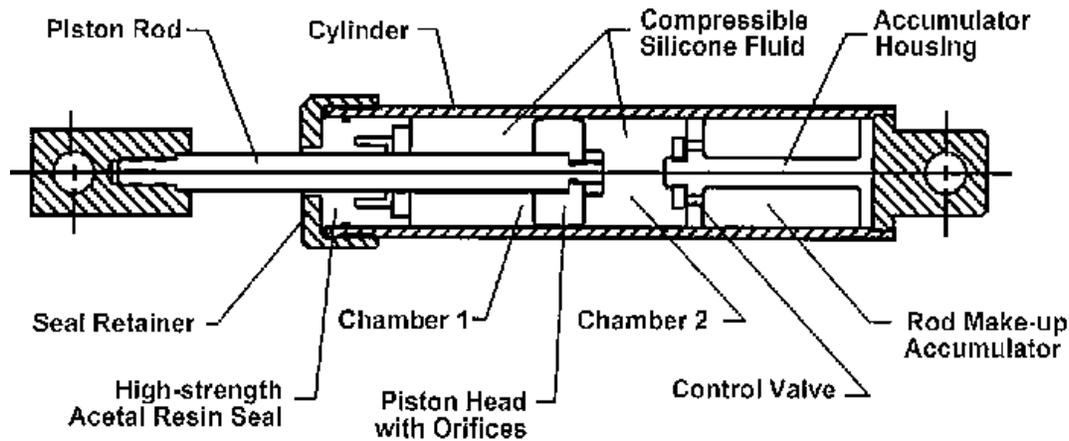
**Commonly used types of seismic dampers include:**
