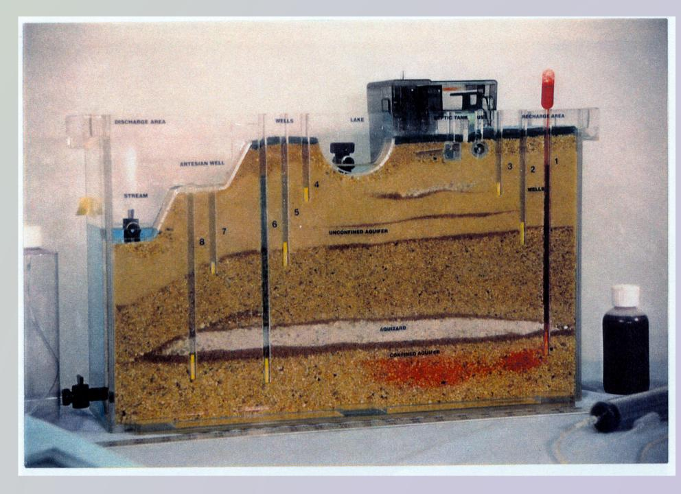
The groundwater model (Crystal Scientific, L.L.C., \$800) simulates the groundwater cycle. It includes a geologic cross-section through three main aquifers, several "wells", recharge area simulated by an aquarium pump, and a discharge area through spigots in a lake and a stream.
