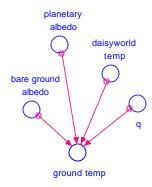
According to Watson and Lovelock's equation 6, local temperature of white and black daisies or of bare ground  $(T_1)$  is a function of planetary temperature  $(T_d)$ , the difference in albedo between the local area  $(A_1, i.e., white or black daisy or ground albedo)$  and the planetary albedo (A), and a factor q that determines whether heat can be conducted from areas of high heating to low heating:
