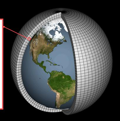
A supercomputer solves all the equations, passing results to neighboring boxes and calculating the next set of initial conditions
