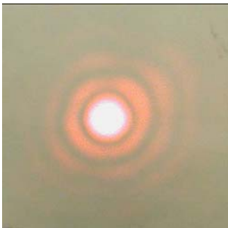
Figure 2. Output of the spatially filtered HeNe laser beam. The spatial filter filter was 10 \mu\text{m} and the magnification of the objective was 20x ( f = 8\text{mm} , \text{NA}=0.4 ). The diffraction limited spot size after the objective was 12.36 \mu\text{m} , so the output power in the central lobe was 22.8% of the input power. The pinhole in this photo was chosen to be somewhat small to show the diffraction rings. A properly filtered beam is a smooth, nearly Gaussian profile with no visible features. Rings like those shown can occur with a properly-size pinhole when the pinhole is not at the focus of the objective. (Courtesy of Basic Skills Lab from Dr. Steve Cundiff and Edward McKenna at the University of Colorado).
