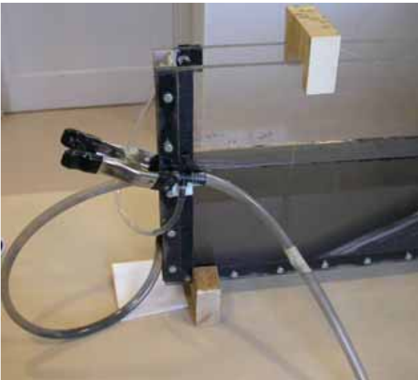
base-level control clipped to tank
