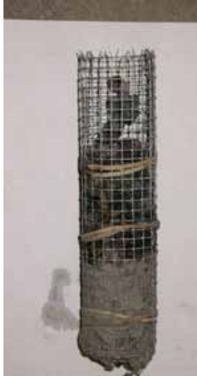
Close-up of sediment diffuser (note that in this photo, bottom of diffuser is covered in sediment; which it won't be, of course, when you initially construct yours.)
