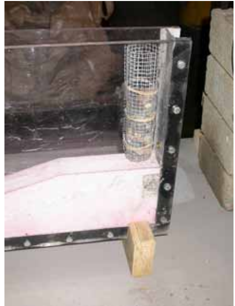
Close-up of sediment diffuser (note that in this photo, bottom of diffuser is covered in sediment; which it won't be, of course, when you initially construct yours.)
