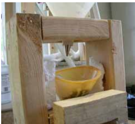
Detail of funnels in stand, showing frosting tip protruding from upper funnel and Styrofoam wedging lower funnel into place in stand
