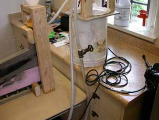
Flow-rate control between pump and head tank
