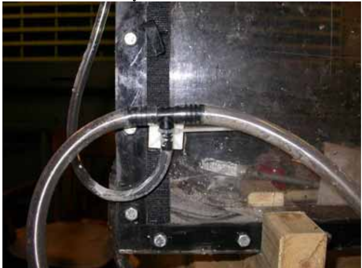
close-up of base-level control, showing 3-way valve
