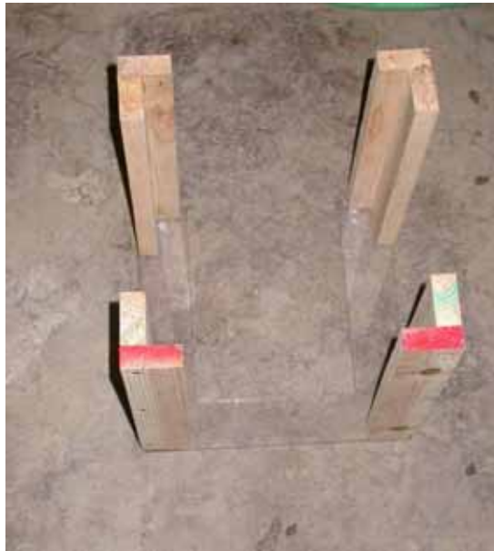
support inverted to show plywood assembly
