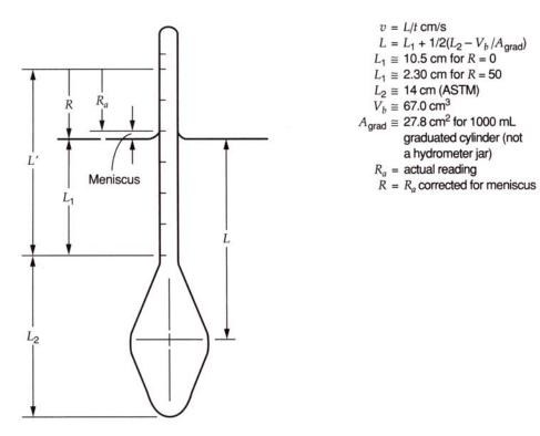
Figure 1. Dimensions of the ASTM 152H hydrometer (from: Bowles, J.E., 1992, Engineering Properties of Soils and Their Measurement, Fourth Edition: McGraw-Hill, New York, 241p.
