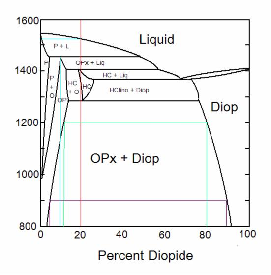
Above is a simplified temperature-composition phase diagram for the system enstatite  $(Mg_2Si_2O_6)$  - diopside  $(CaMgSi_2O_6)$ , which are common constituents of peridotites, gabbros, and basalts. The phase abbreviations are:
