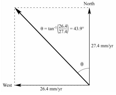
In this case, the station is moving  $43.9^{\circ}$  to the west of north, or toward an azimuth of  $(360^{\circ} - 43.9^{\circ}) = 316.1^{\circ}$ .
