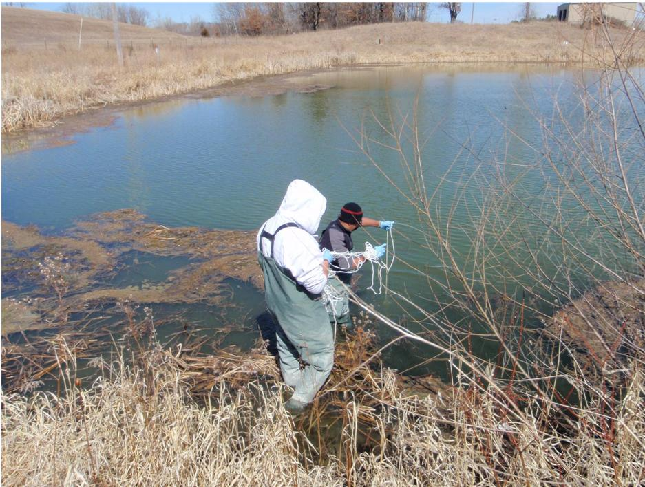
Students deploying a grab sampler to collect surface sediments from the sedimentation pond.
