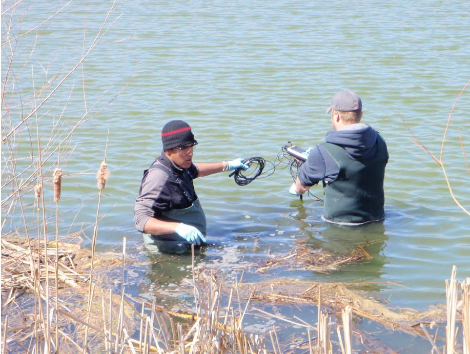
Students making measurements in a lined sedimentation pond at the base of the cascade aeration system.
