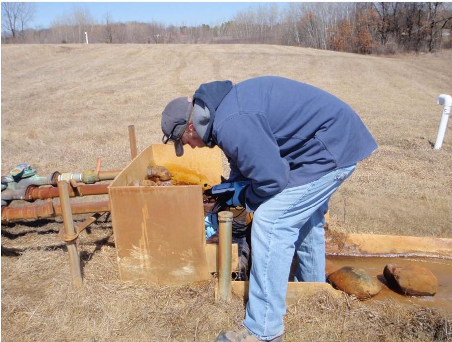
Student making measurements at the top of the cascade aeration system.
