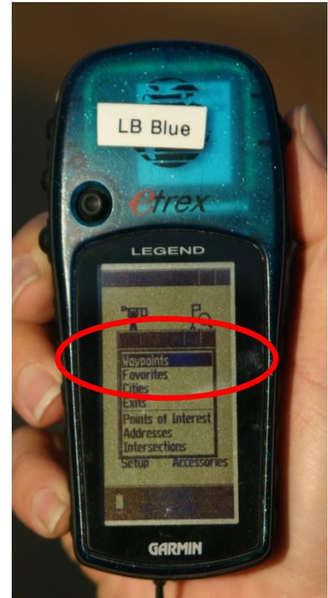
1. Turn GPS Unit on, hold button in until display activates.
