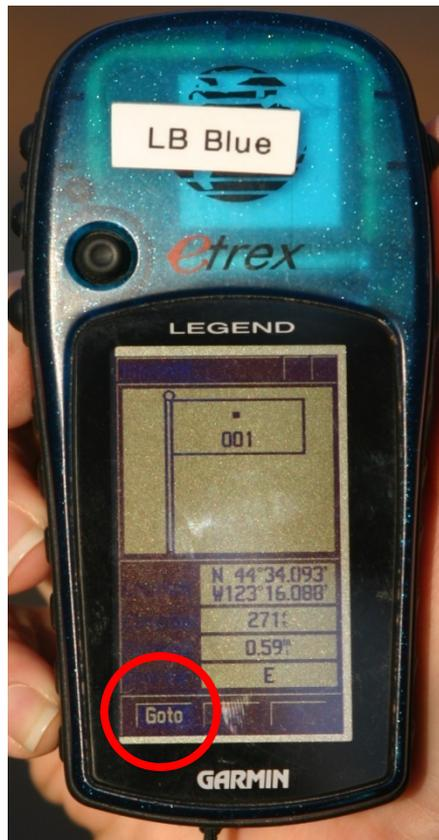
9. Use the Toggle Button to highlight ‘GoTo’ function, moving up/down or right/left
